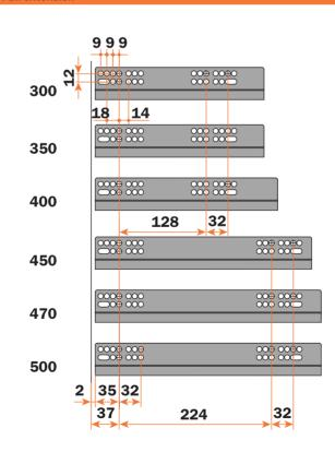
For the function Push is required a A value = 2,5 mm.
