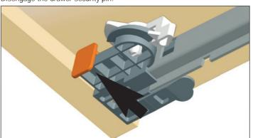
Lift and disengage the drawer.
