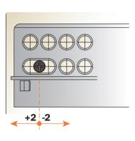
The oval slot allows the easy alignment of drawer frontals particularly in multi drawer and Push applications.
