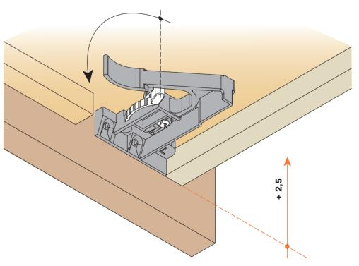
Drawer height adjustment (+ 2,5 mm) using the lever indicated
